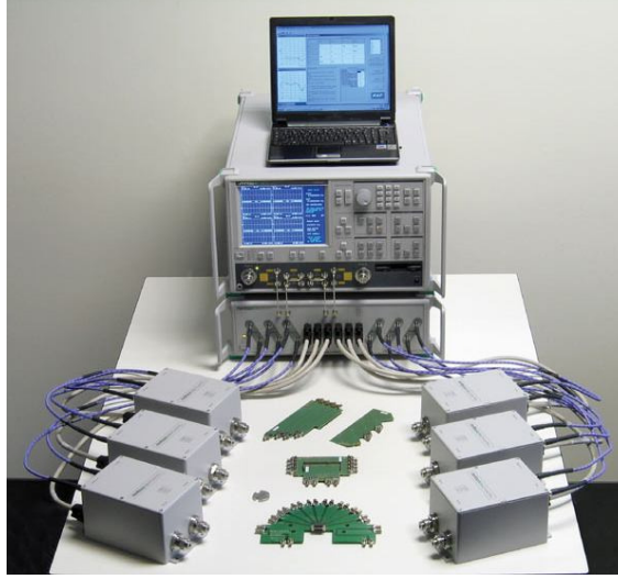
Figure 2.7. The 12-port ( N + 2 )-samplers Anritsu 37397D VNA has 40 MHz to 67 GHz frequency range. The system consists of a 37000D-family two-port VNA (top) coupled to an extension box (bottom) that contains the port switches and auxiliary power supplies. The measurement couplers are contained in six modules (two port each), which are placed as close as possible to the DUT in order to minimize high-frequency losses. The measurement and calibration software runs on an external computer. Courtesy of Anritsu [5].
